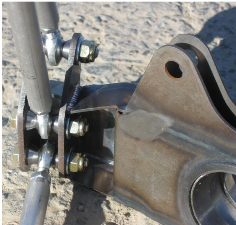
Figure 43: Front (High Camber) Lower Control Arm Pivots, Steering Pivot, and Heim Joint Spacers
