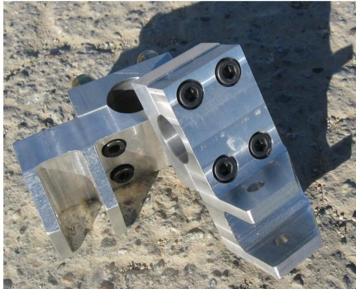
**Figure 39: Anti-Bumpsteer Steering Rack Clevises**
