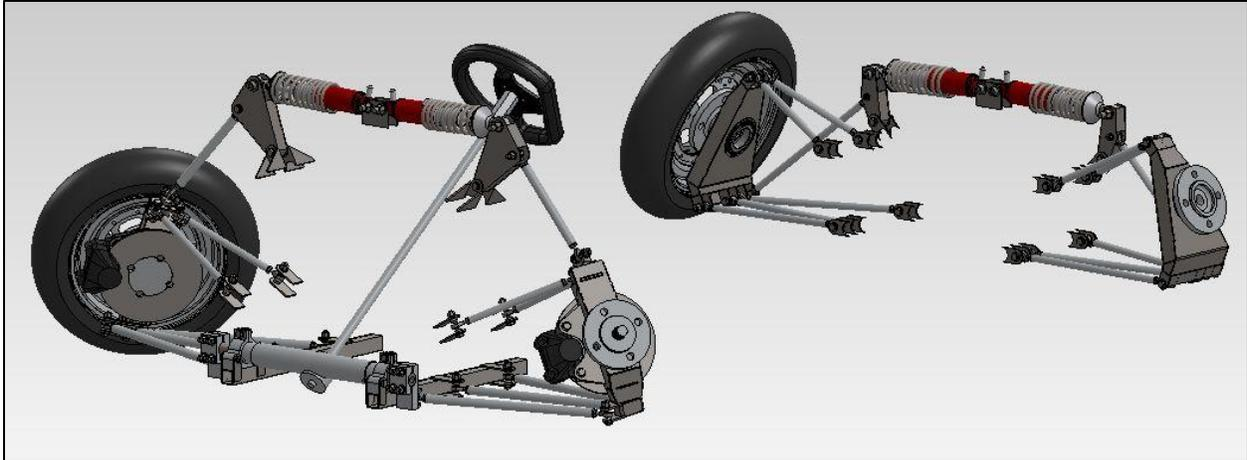
Figure 37: Final Suspension Design
