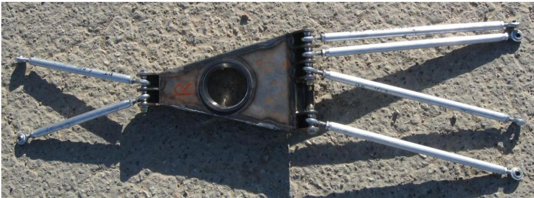
Figure 38: Right Rear Suspension Corner
