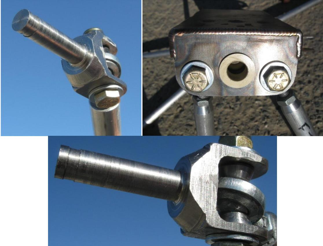
**Figure 40: Front Pushrod Rotating Clevis and Bushing Area**
