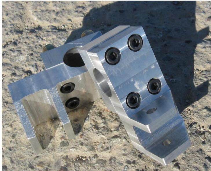
**Figure 39: Anti-Bumpsteer Steering Rack Clevises**
